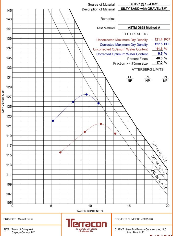
ABORATORY TESTS ARE NOT VALID IF SEPARATED FROM ORIGINAL REPORT. COMPACTION - V1 J5206196 GARNET SOLAR FIELD INFO 2-12. GPJ TERRACON DATATEMPLATE.GDT 2/12/21
