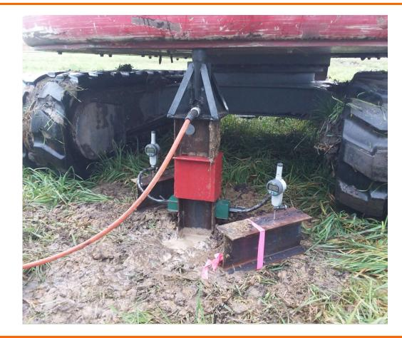
Photo 5: Compression load setup and deflection measurements (Typical)
