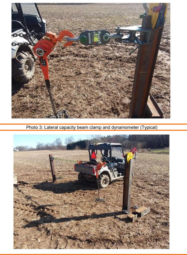
Photo 4: Lateral capacity setup (Typical)
