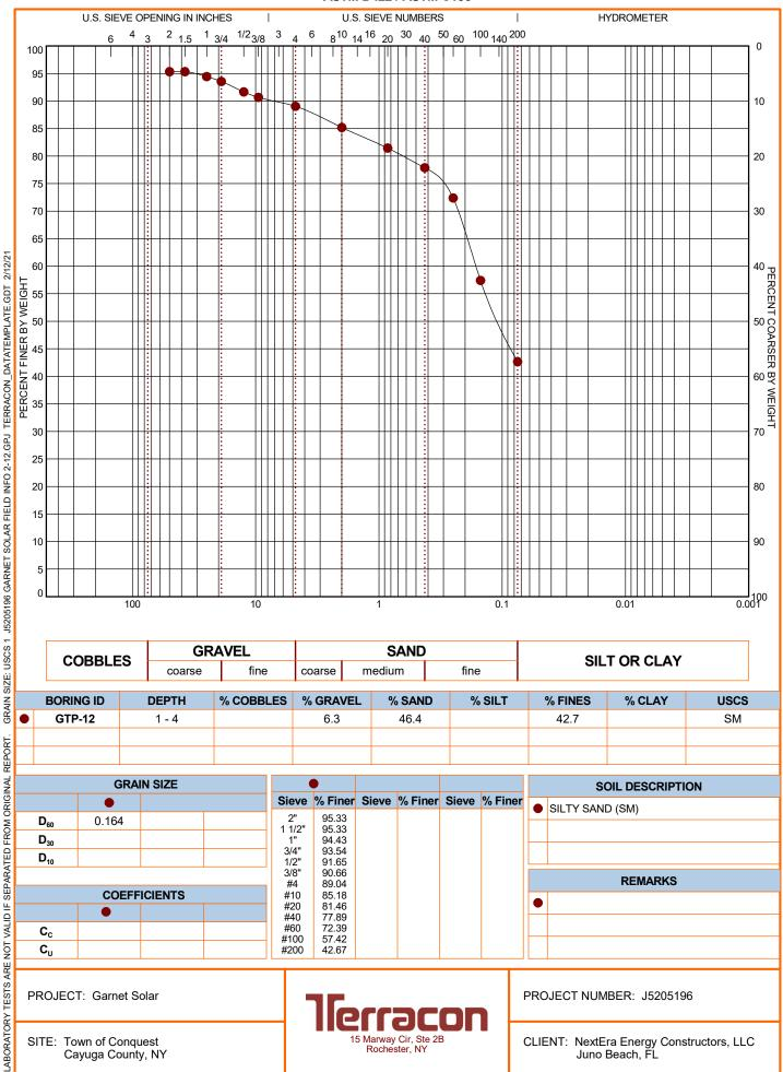
GRAIN SIZE DISTRIBUTION ASTM D422 / ASTM C136
