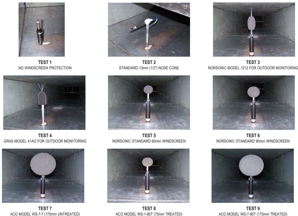
Fig. 2—Photographs of nine microphone test configurations.
